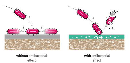
An anti-bacterial lacquer gradually releases slowly diffusing activeing redients. These not only prevent the bacteria cells from dividing, but destroy them permanently. Bacteria reduction of up to 99% in 24 hours.
