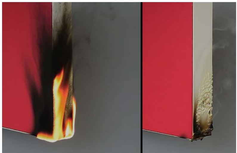
Comparing a conventional edgeband to RAUKANTEX FP
