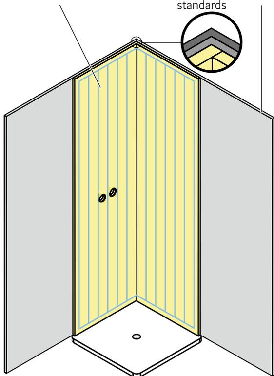
Due to joints and connection points on surfaces that are directly exposed to moisture, this requires the installation of additional sealing (sealing membranes or liquid sealants) under the wall covering. The stress classes for moisture exposure as defined in DIN 18531 must be taken into account.
