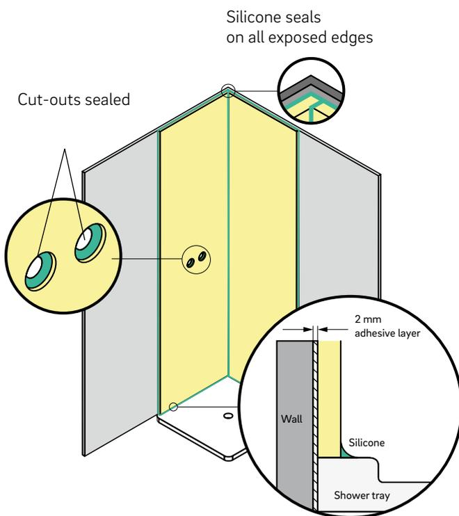
To seal the outer and abutting edges, REHAU recommends silicone grouting across all exposed edges to prevent the ingress of moisture, dirt, waterlogging and mold.
