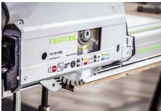
The quality of the cut edge depends on the tooth shape, the number of teeth on the saw blade and the cutting speed.
