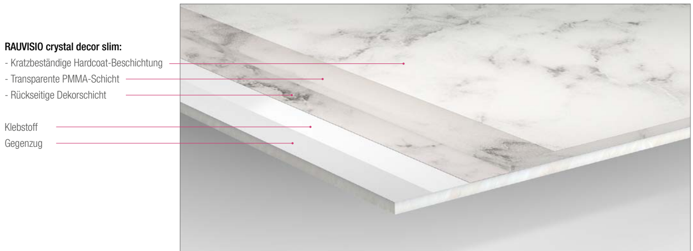
Abb. 7-2 Systemverbund RAUVISIO crystal decor slim
