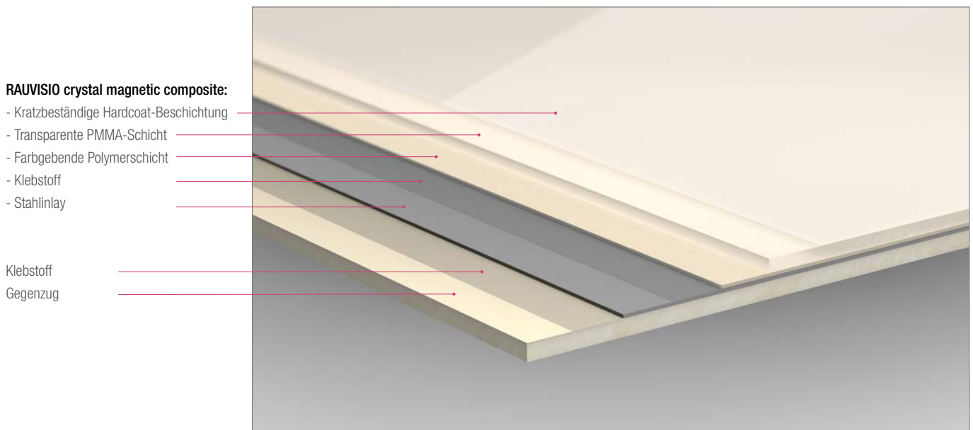
Abb. 4-2 Systemverbund RAUVISIO crystal magnetic slim
